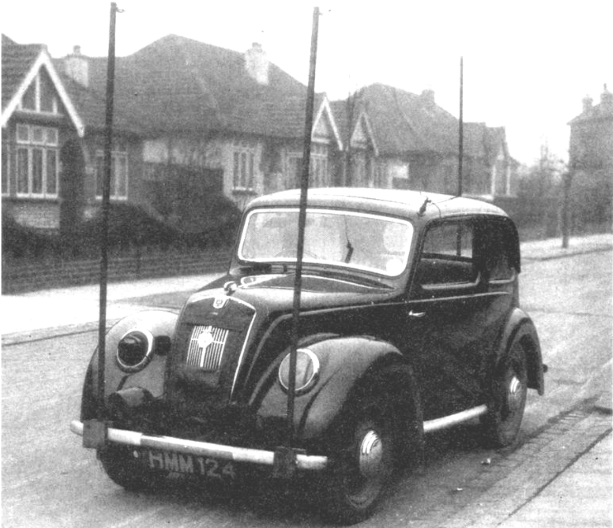
HF Mobile -- detail unknown but at a guess during WW2 due to the muted headlights. Note the antenna feed point.
