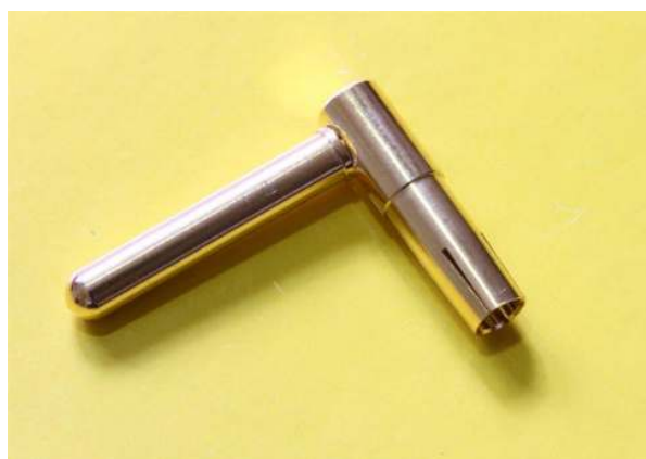
Roger ZS6RJ sacrificed R63.- to inspect this one. Note the solid reliable connection that should not give any trouble.
