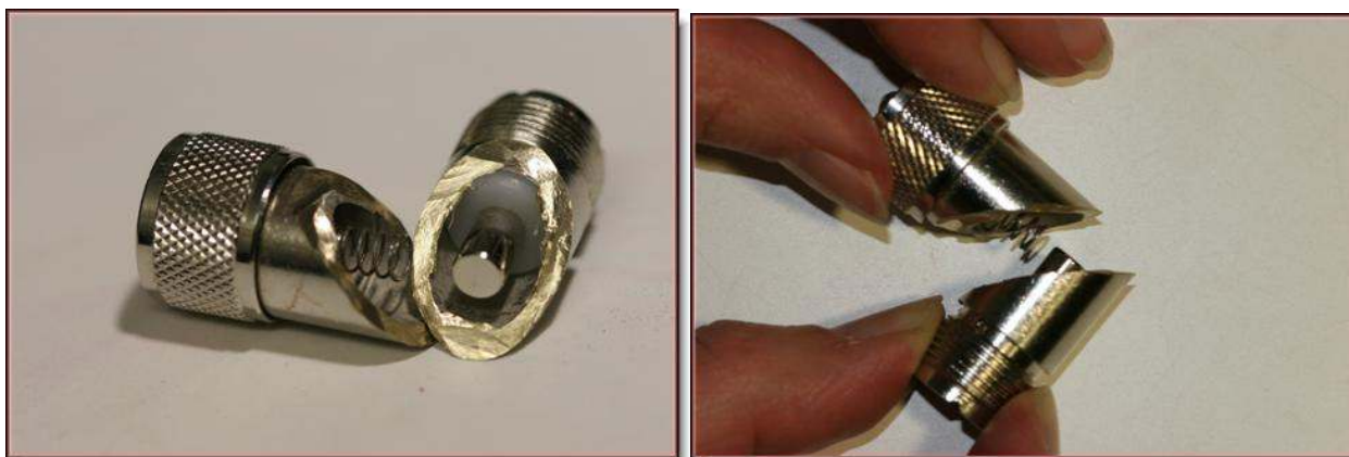
ZS6BAQ opened a R20.- Taiwan elbow. Note the inductive/variable R coupling! Some stock were even open circuit!
